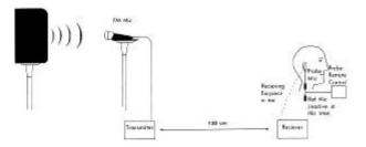
Fig. 5: Physical arrangement for probe microphone measures of an FM system in the FM mode of operation. (Adapted from Frye Electronics, 1993. Used with permission)
