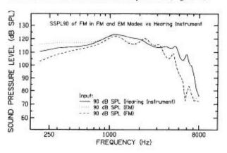
Fig. 4: Coupler SSPL90 of an FM system in FM and EM modes of operation compared to a hearing instrument.
