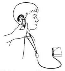
Fig. 2: Physical arrangement for coupler measures of an FM system coupled to a personal hearing aid via a neckloop. (Adapted from Frye Electronics, 1993. Used with permission)
