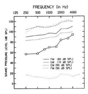
Fig. 6: Real ear sound pressure level measures of an FM system in the FM and EM modes of operation for an individual with a moderate to severe hearing loss.
