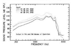
Fig. 3: Coupler *output* of an FM system in the FM and EM modes of operation.
