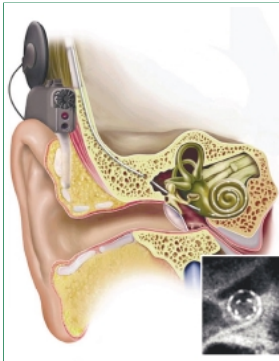
Figure 6: All cochlear implants share key components, including a microphone, speech processor, and transmitter coil, shown in a behind-the-ear position in this diagram
